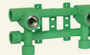
The fittings are manufactured in accordance to DIN 16962 from Polypropylene Random (Type 3) and available in diameters from 20mm up to 450 mm. For the production of the fittings the company uses raw material with a low melt flow index, identical to that of its pipes, so that the mechanical strength of the pipe does not differ from that of the fittings. They are produced with a wall thickness equivalent to 30 bar.
